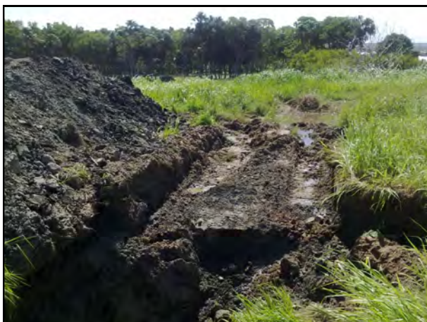
Photo 5: Test pit in former Disposal Pond 17/02/11
